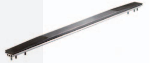
The current distribution factor is used to adjust the current distribution between several strips which are mounted on the same pantograph. The first strip gets more current than the others and we have to choose the grade according to this unfavorable situation. For example, with 2 strips, the first one gets 60% of the total current on the pantograph.
