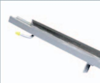
This device enables the pantograph to be lowered if an impact severe enough to damage the pantograph head was to occur.
