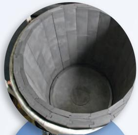
Graphite & insulation equipment for Siemens CVD process
